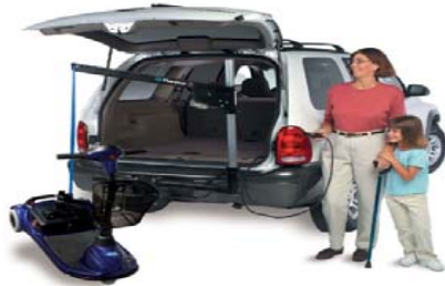
Inside lift for power mobility device
